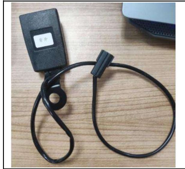
Figure 2-37 Seat Belt Switch Diagram
